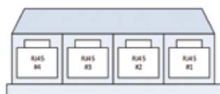
#1: Ethernet port 1 #2: Ethernet port 0 #3: RS485/RS422 #4: RS232
